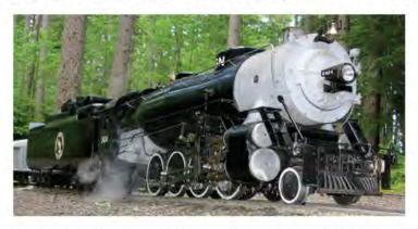
2-8-2 Mikado, 1.6 scale, Great Northern Completed in 1989 by Bernie Swenson from Little Engines design. New ASME steel boiler with copper tubes in 2003, steel clad drivers, Super scale fittings. Propane fired. Engine weighs 1260 lbs wet. Tender: 6 wheel equalizing trucks with stainless steel water tank and twin 5 gallon propane tanks, 650 lbs wet. Heavy duty stands and spare tanks included. Engine has effortlessly pulled 43 people around the KLS Track. Has been to TM many times.
