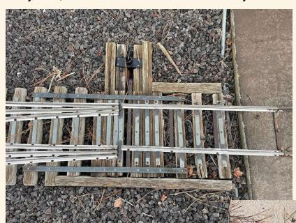
a gap in the switch of as much as two inches. The 24 switches were rebuilt, with new rails, and are now attached to the turntable. They should last another 30+ years. Hopefully you can tell the "before" and "after" pictures. I had help from Gil Dominguez, Tom Watson and Ron Domoe.
