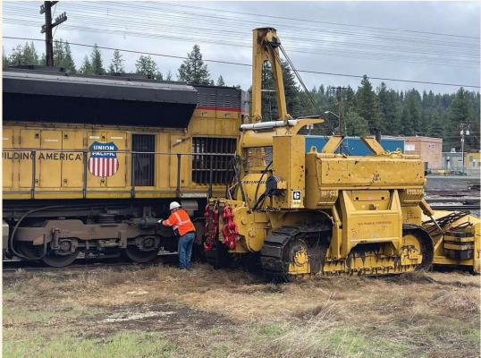
replace with an axle without a motor. The locomotive would be sent to a repair facility where a new motor would be installed
